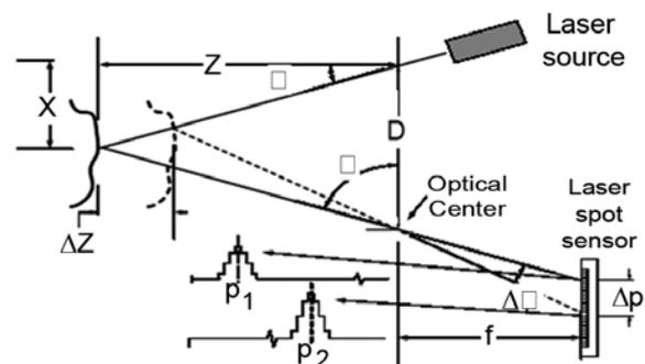
Fig. 6 - Triangulation-based laser scanner principle scheme.
