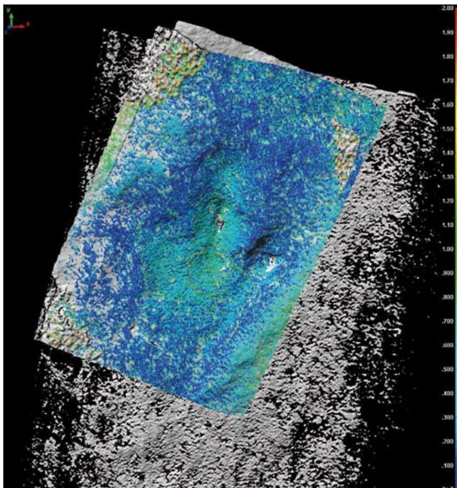
Fig. 15 - Colour-coded difference between the laser scanner and photogrammetric models. Note as in the track area the difference between the two models is on average less than 1 mm.
