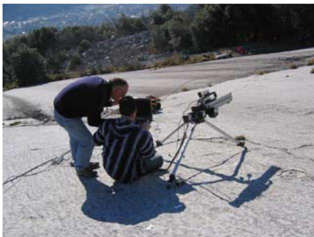
Fig. 7 - Laser scanner ShapeGrabber SG1002.
