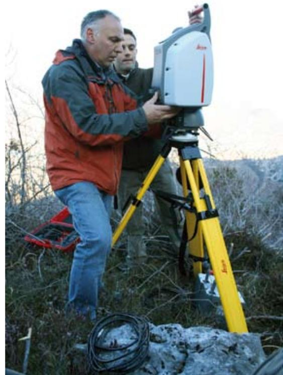
Fig. 3 - Leica ScanStation 2 laser scanner used for the acquisition of the data.
